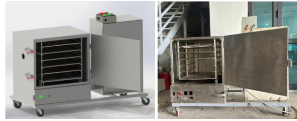
[Fig.3: 3D View and Actual Physical System of the Hybrid Heat Pump Drying System Integrated with Electric Heating]
