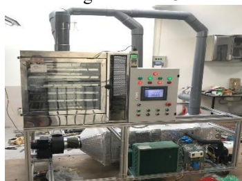
[Fig.2: Actual View of the Heat Pump Drying System Used in the Experiment]
