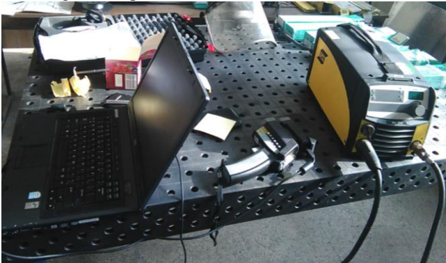
Fig. 4. Contactless IR temperature measuring device Raytek MX6 with a K – probe thermocouple
